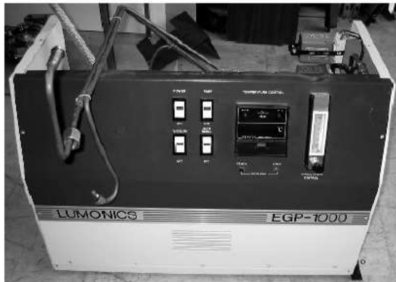
Figure 7: Cryogenic gas processor.
