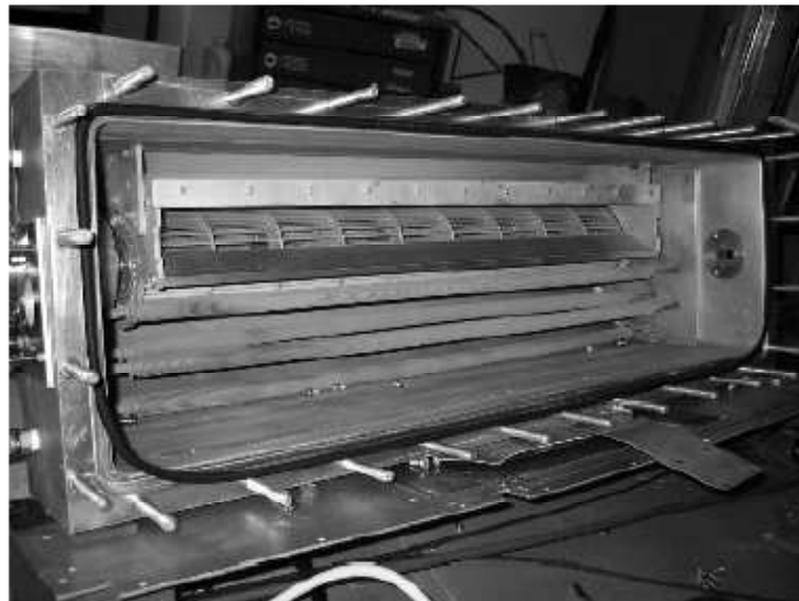
Figure 11: Excimer laser heat exchanger and fan.
