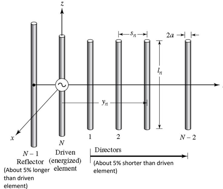
**Fig 2:** Typical Yagi-Uda antenna configuration.
