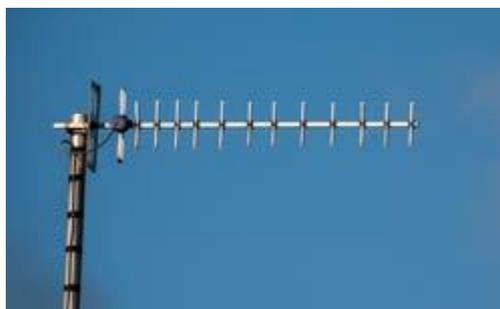
**Fig 1:** Yagi-Uda antenna showing element types.
