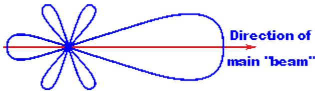
**Fig 3:** Yagi-Uda antenna radiation pattern.
